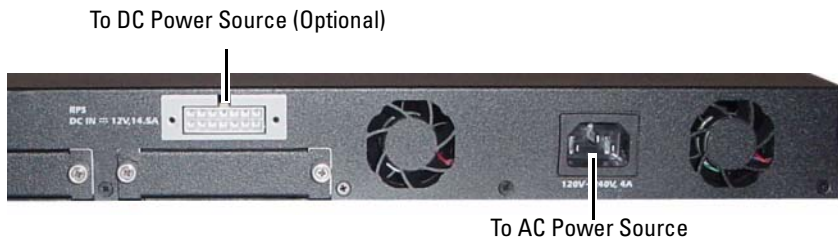
Figure 1-15. AC and DC Power Connection to Switch
